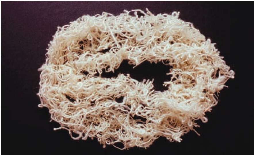
3: Sample of high-twist yarn after wetting out, showing contraction and spiraling of the yarn.
