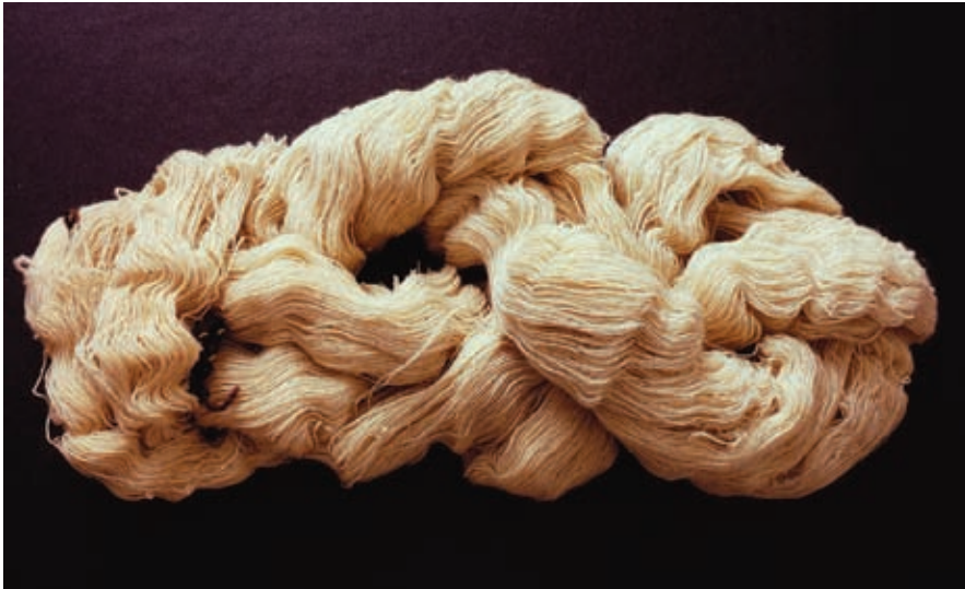
2: Skein of high-twist yarn. The strain energy stored in this yarn will not become obvious until the yarn is wetted out.
