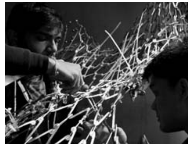
Fig. 2.1.5 Assembling the laser cut aluminium components of a lily
