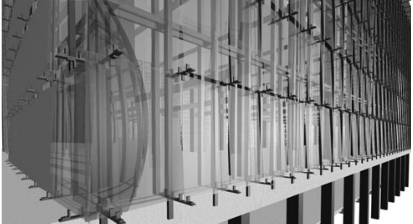
Figure. 2: Façade detail, Canadian Embassy in Berlin, digital model by Peter Marshall, University of Waterloo, 1998
